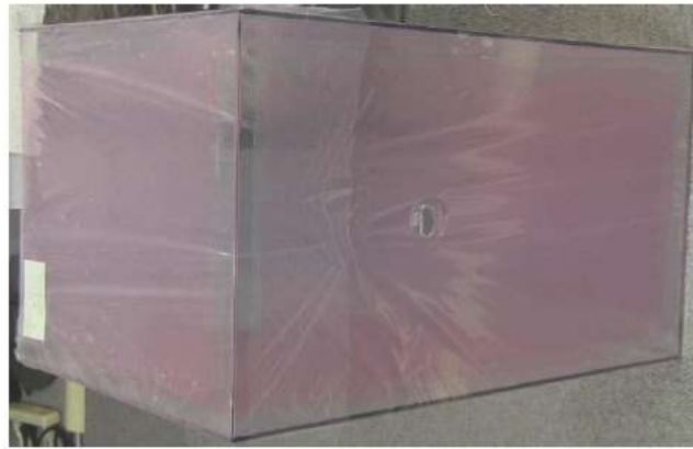
Figure 12. Photo of the acrylic calorimeter enclosure.
