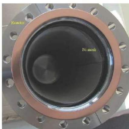
Figure 3. View of Ni mesh in the reactor.
