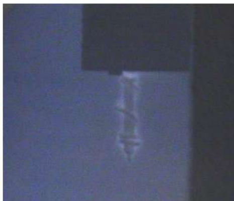
Figure 7. Photo of plasma state in which a high voltage is applied to the Pd thin wire on the ceramic heater.
