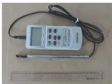
Figure 15. Air volume measurement tool for calibration.
