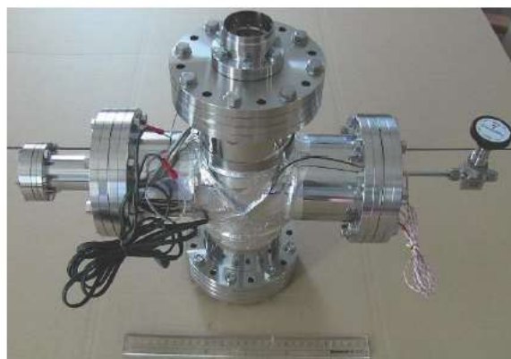
Figure 1. Photo of the reactor body. The upper part is the electrode inlet part, on the left is the viewing window, and the gas valve is seen on the right. A heating wire is wrapped around the reactor body center part. The connecting wire and platinum temperature sensor can be seen.
