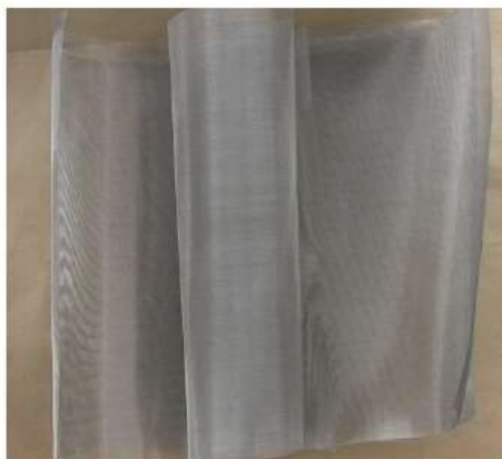
Figure 2. Nickel mesh as reactant, 30 cm 2 , 200 mesh. This photo shows the two meshes overlapped.
