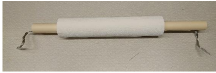
Figure 4. The Mini Superthal heating element with an Alumina reactor tube inserted inside the coil. The metal strings are connections to the solid coil inside the fiber cylinder.
